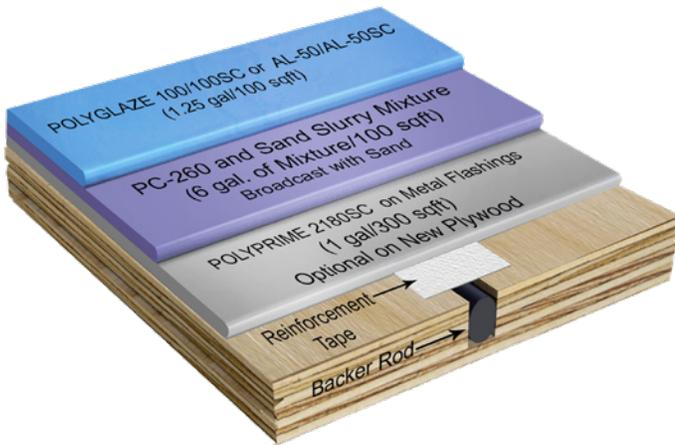
Plywood Substrate System with Sand Aggregate
